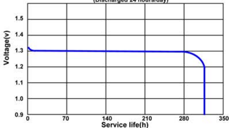
DISCHARGE CHARACTERISTICS AT 620Ω 25°C 60%RH (Discharged 24 hours/day)
